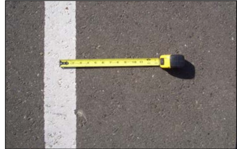
measure to center of painted stripes
