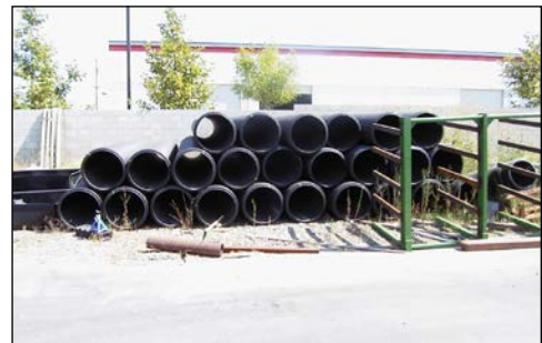
circular pontoons to be foam filled
